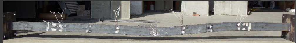
Top view of self-reacting test frame (above) and deformed column specimen(below).
